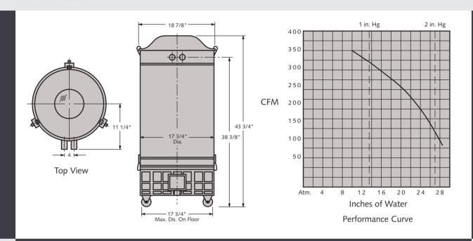
Model SR 400 Max. Differential Pressure  $28.5" H_2O$
